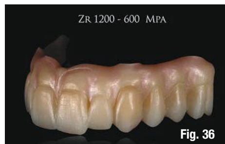
Figs. 35 - 37: Zirconia "Multilayer" Multichromatic 1300 MPa, sintering temperature 1550°C, Microwave process in 4.00 hours.
