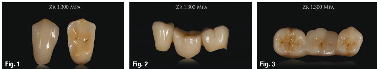
Figs. 1-3: Zirconia "Multilayer" Multichromatic 1300 MPa, sintering temperature 1550°C, Microwave process in 4.00 hours.
