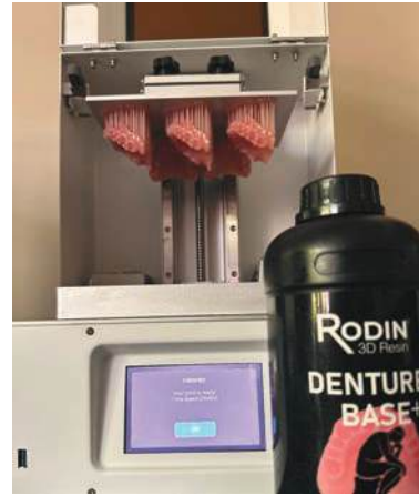
FIGURE 7: The Phrozen printer is fast and reliable, with a larger print platform for production, and a large material library. These 5 bases were printed with Rodin Denture Base +
