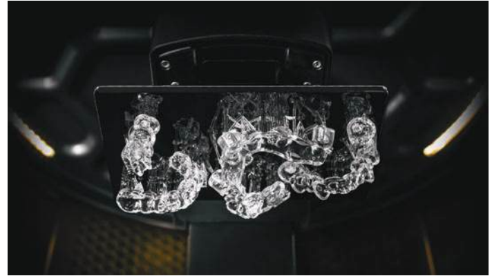
FIGURE 18: Surgical guides are essential for precise implant placement, whether it's a single crown or an all-on-X procedure. The Carbon printer streamlines the process by handling multiple prints at once, allowing technicians to focus on other critical tasks and save valuable hands-on time.
