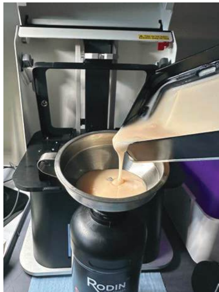
FIGURE 11: All materials should be siphoned through a funnel with a screen mesh to separate cured resin and debris. These are sold on Amazon for about 12 Dollars US.
