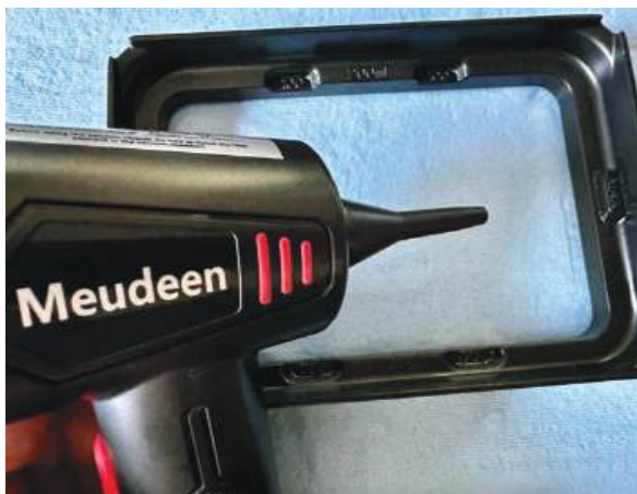
FIGURE 13: Blow dry the resin Vat with a rechargeable Blower-Vacuum. Also purchased from Amazon for about 24 dollars US.
