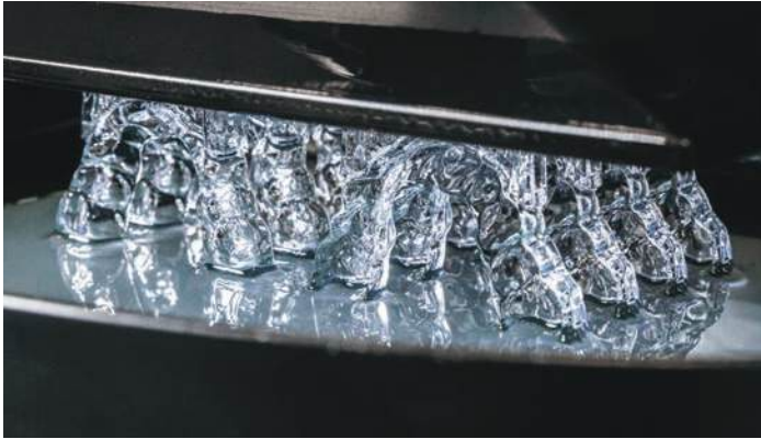
FIGURE 17: Night guards offer significant profitability, by efficiently producing a large volume of high-quality prints in a single run on the Carbon 3d printer
