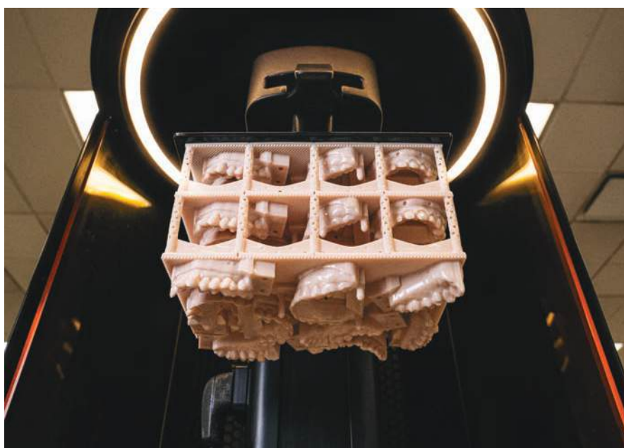
FIGURE 16: The Carbon printer is an exceptional choice for large laboratories, offering the ability to stack models for increased efficiency. This feature, also available on other printers, makes it a versatile option for scaling production.
