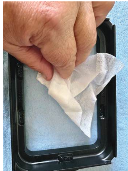
FIGURE 12: Clean the resin Vat with an Alcohol wipe after whipping out excess resin with a lint-free absorbent disposable towel.
