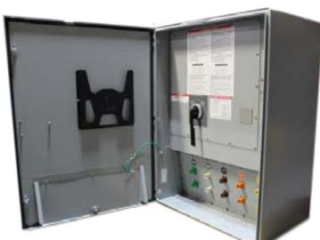
The Breaker Series Docking Station contains an integrated circuit breaker within the unit, available up to 600VAC. These units are thermal magnetic breaker standard (electronic available). This series is more commonly used when a breaker or switching device isn't directly connected down stream.
