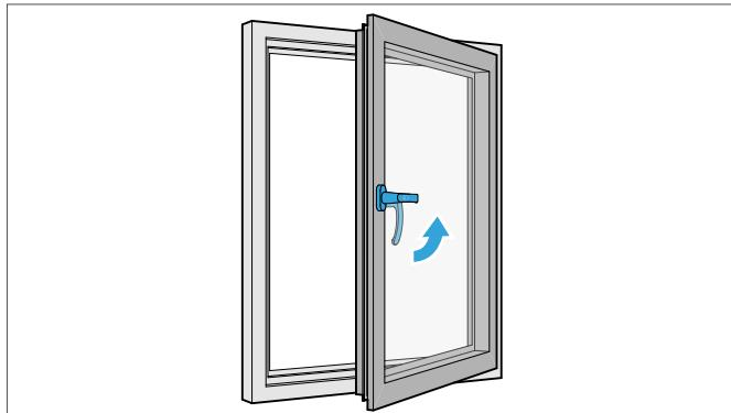
2. Push the element sash further open or closed.
