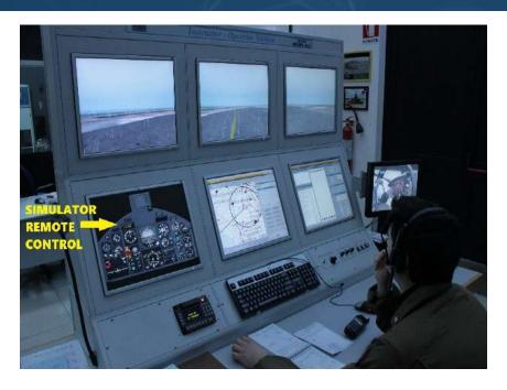
The Instructor could control the simulator and interact with the pilots.
