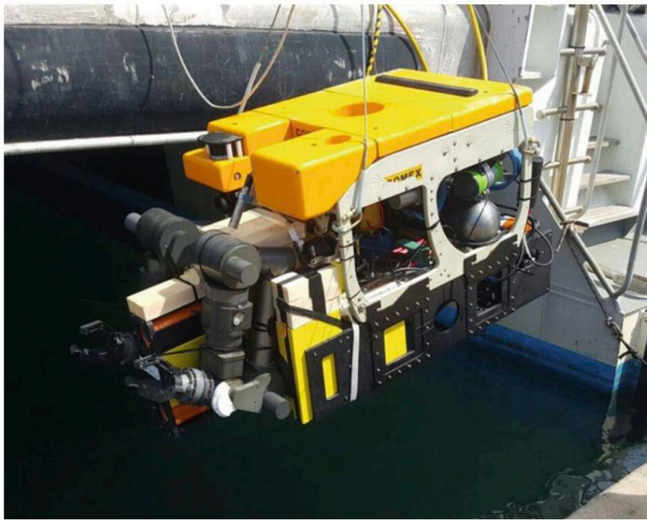
Fig. 1.13 The DexROV vehicle on the crane in the configuration with two 6-DOFs arms (courtesy of Jeremi Gancet, Space Applications Services, Peter Weiss, Comex, Alessio Turetta, Graaltech and DexROV Consortium)
