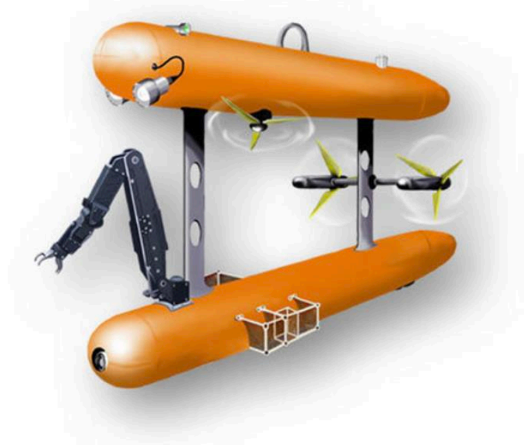
Fig. 1.9 Proof of concept for a Woods Hole Oceanographic Institution vehicle equipped with a manipulator, named Jaguar (courtesy of H. Singh)
