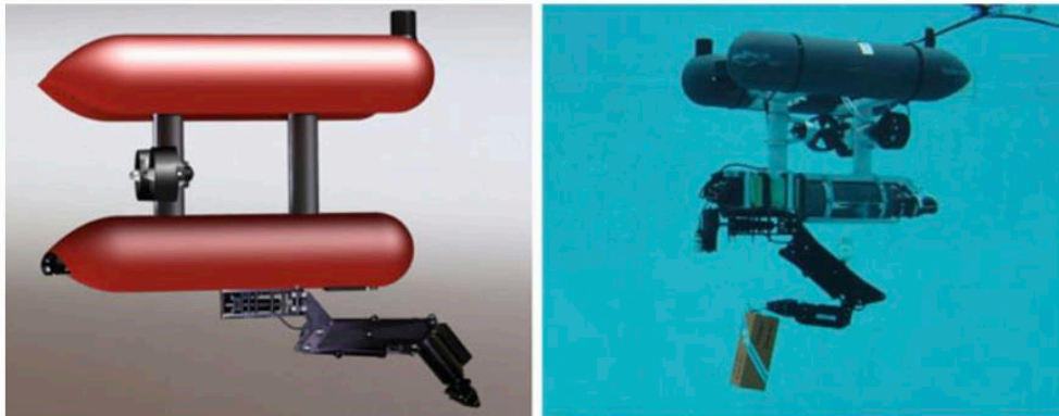
Fig. 1.10 Girona500 equipped with a CSIP arm developed at the University of Girona (Courtesy of Pere Ridao, Centre d'Investigaci3 en Rob3tica Submarina (CIRS), Computer Vision & Robotics Research Team (VICOROB), University of Girona)
