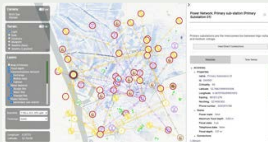
The image shows how Anglian Water's assets, UK Power Networks' electricity distribution assets and British Telecom's communications assets are interconnected.
