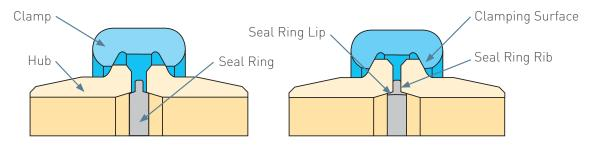
Rib of the seal ring is clamped between hub faces. Lips of the seal ring engage inner hub surfaces in an interference fit that deflects the lips to achieve a seal
