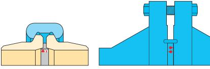
Internal pressure energizes the Grayloc® seal lips, reinforcing the seal
