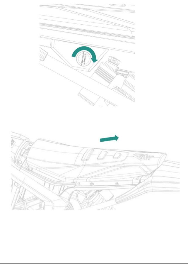
2. Position the battery charging port towards the right side of the frame, place it into the battery compartment, and install the discharge plug (ensure that the ignition switch is in the off position). Close the seat.
