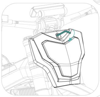
2. Adjust the position as needed, then use a 5# hex wrench to tighten the central securing bolt.
