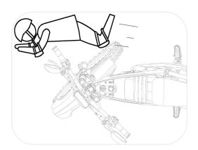
Squeezing the rear brake abruptly with the right foot while riding may lead to a side fall. (For European versions, squeezing the brake suddenly with the left hand)
