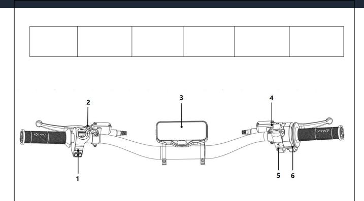
1-Left Assembly Switch 2-Rear Brake 3-Dash 4-Front Brake 5-Right Assembly Switch 6-Right Throttle
