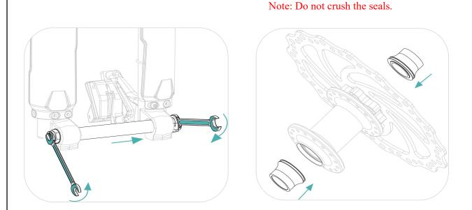
3 . Remove the brake caliper pads, align the front wheel with the front fork mounting position, insert the brake disc into the brake caliper, and use an 8# hex wrench to secure the front axle.
