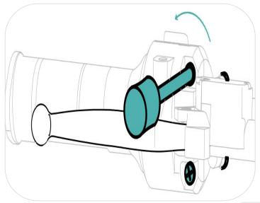
2.As shown in the picture, adjust the throttle to a upward or downward angle of  $5^{\circ}$  for a comfortable grip distance. Use a 4# hex wrench to secure it.
