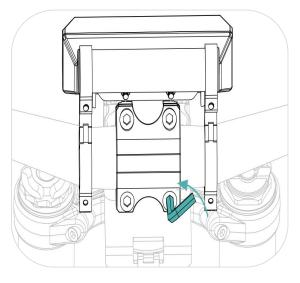
2. Place the riser block and handlebars on the front headlight bracket, aligning the holes, and use a 5# hex wrench to tighten the four screws.
