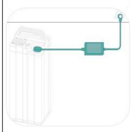
(2) The charger indicator light displays as follows: The red light indicates that it is charging. When fully charged, the green light will remain on continuously. Please turn off the power when the battery is fully charged.
