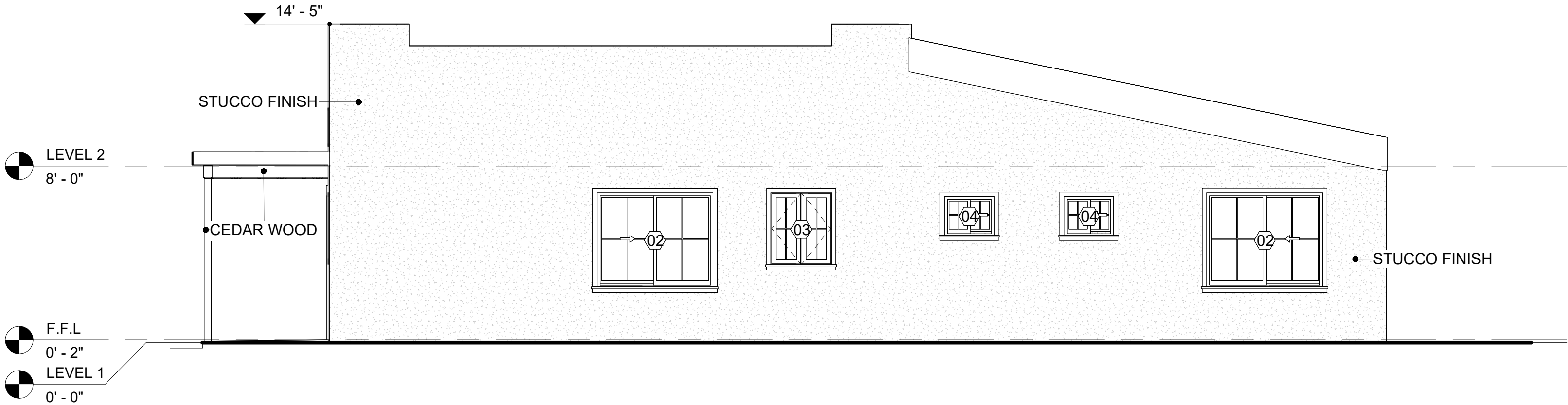
2 RIGHT SIDE ELEVATION 1/4" = 1'-0"
