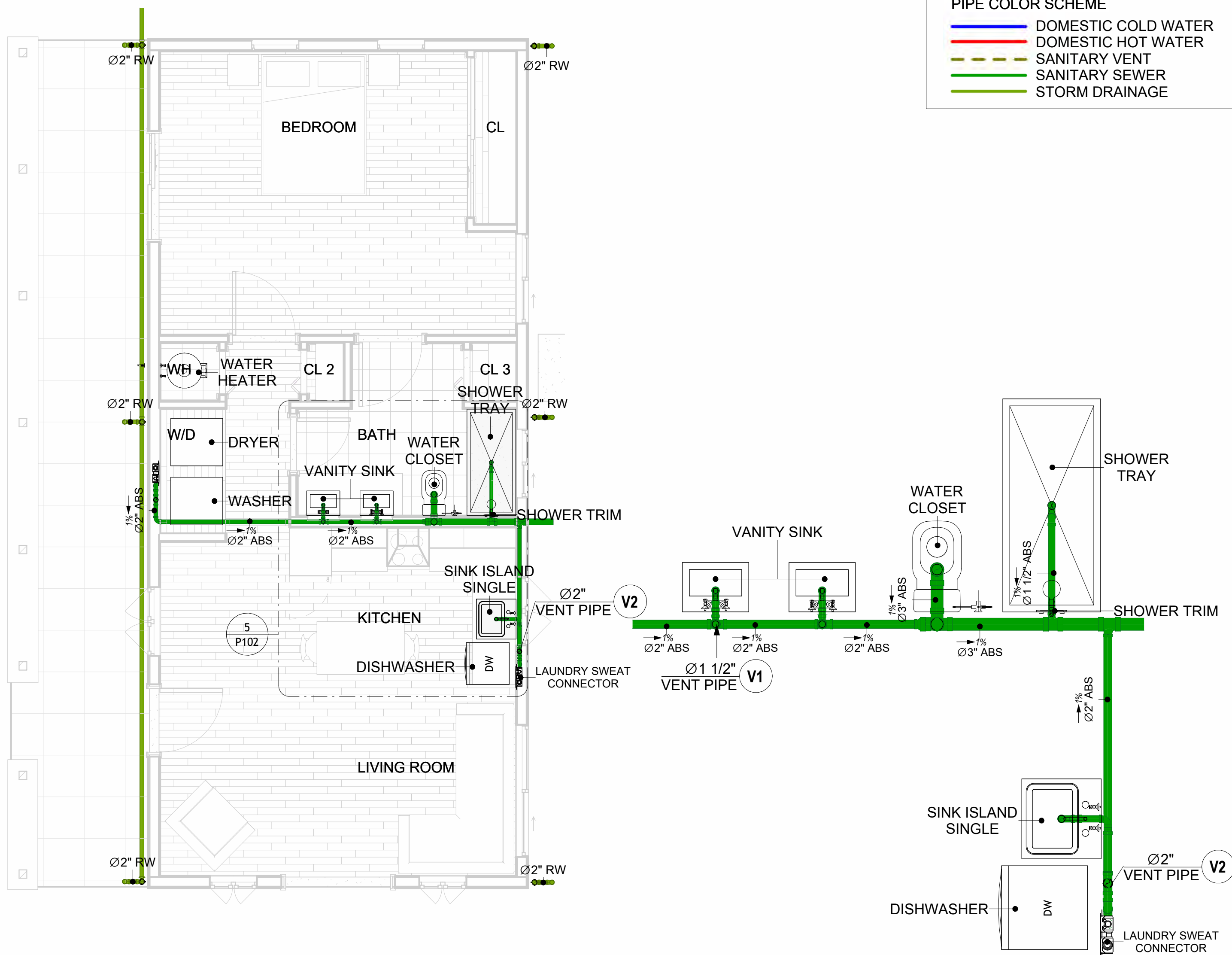
4 OVERALL SANITARY 1/4" = 1'-0" 5 KITCHEN AND BATH SEWAGE 1/2" = 1'-0"
