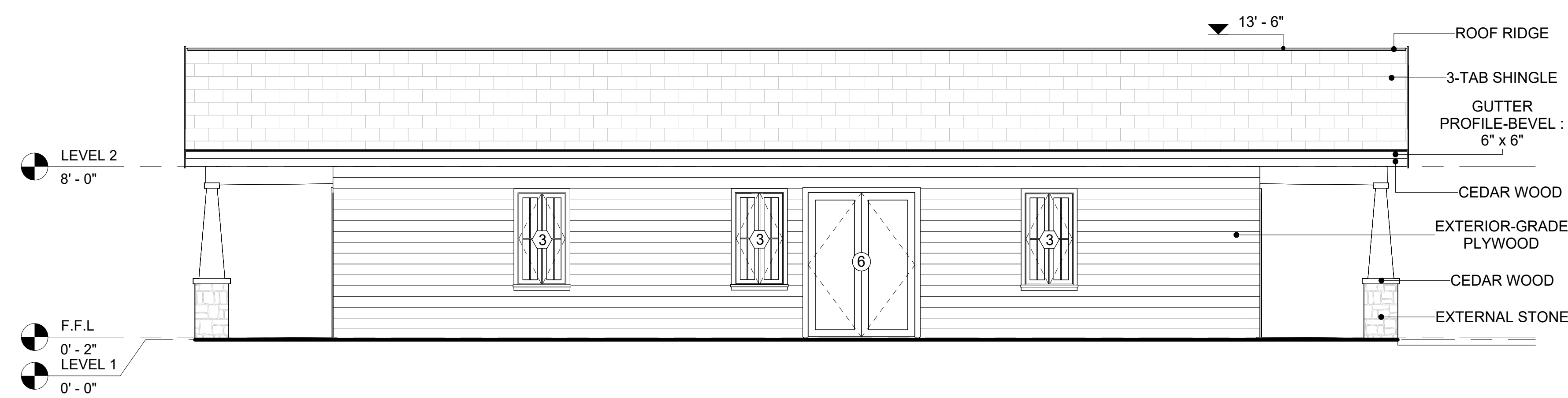
2 LEFT SIDE ELEVATION 1/4" = 1'-0"
