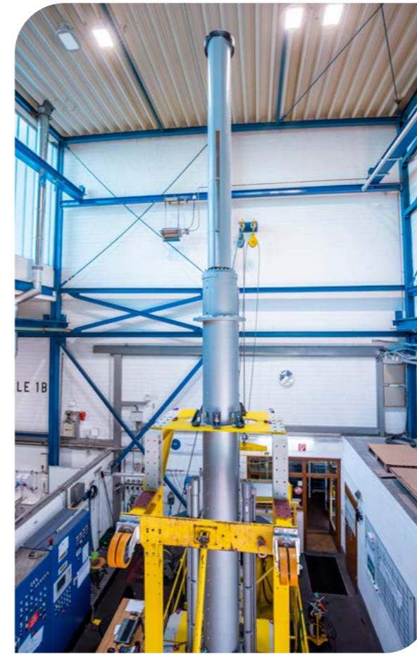
GABLER mast systems are fully integrated, hoistable (extendable) submarine and XLAUV masts that provide mission-critical capabilities for observation, reconnaissance and protection whilst being designed for the lowest possible signature
