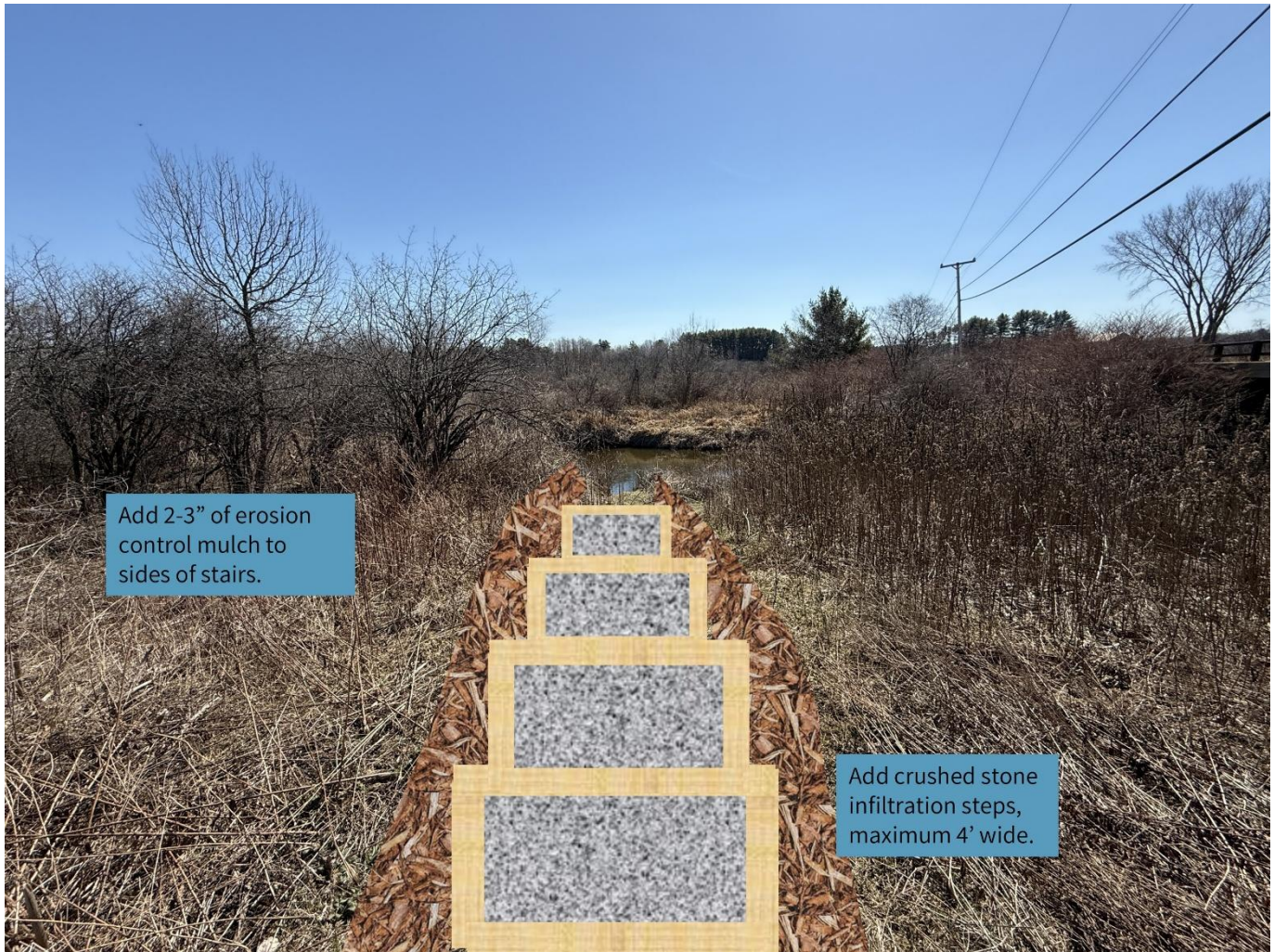
Figure 2. View of proposed infiltration steps from the top of the slope facing the Royal River.
