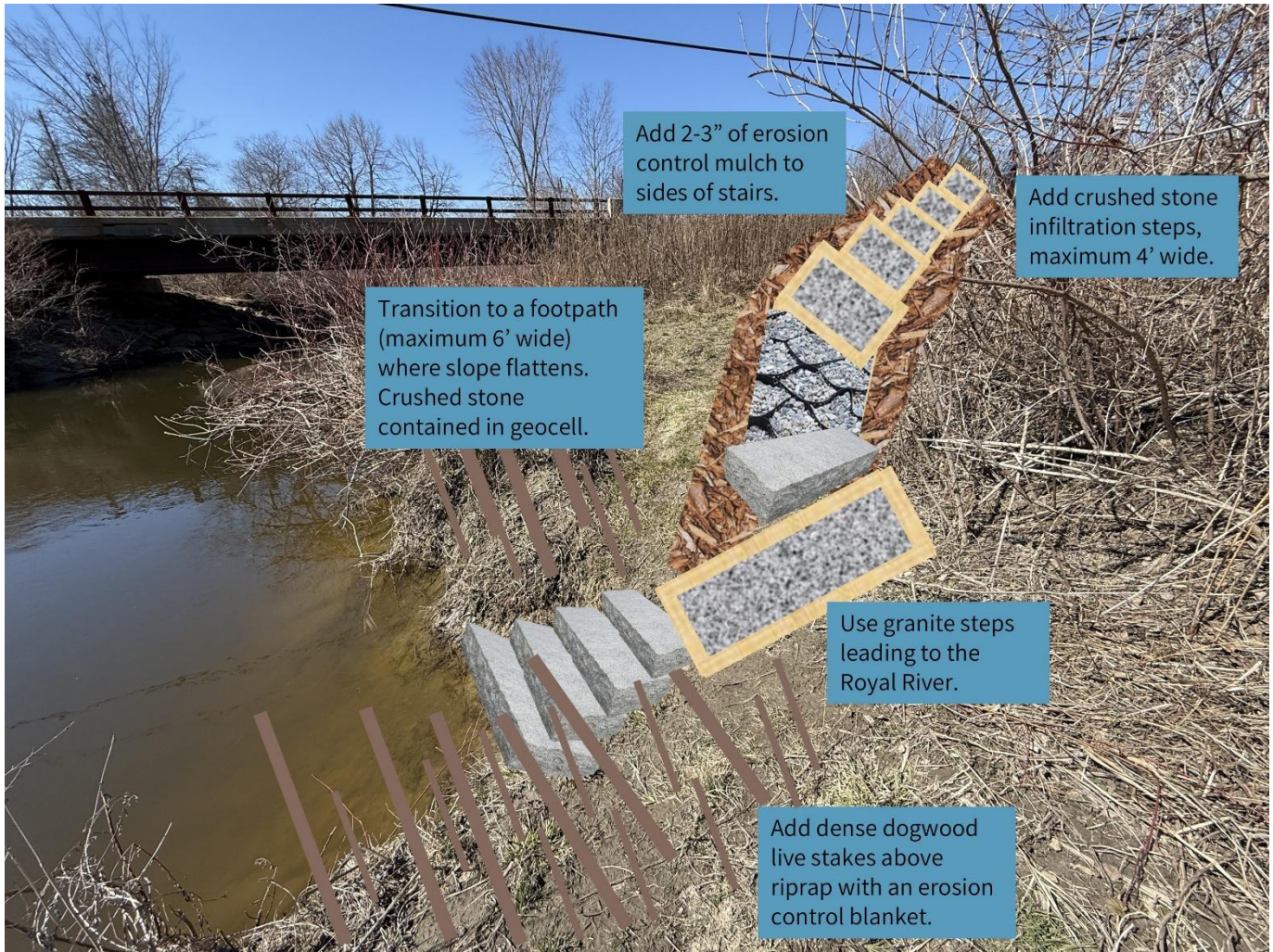
Figure 4. View of the proposed infiltration steps, footpath, granite steps, and dogwood live stakes bank stabilization along the Royal River.
