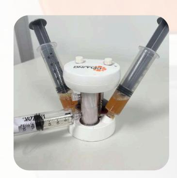
Push the remaining aqueous plasma through the back filter by pressing the plunger of the syringe on Port B. The plasma will be redirected to Port C automatically.
