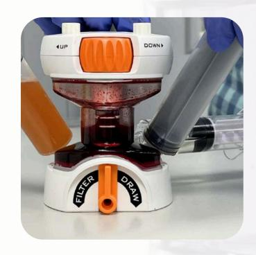
Store the plasma in the Port C syringe, return the flow valve to the neutral position.
