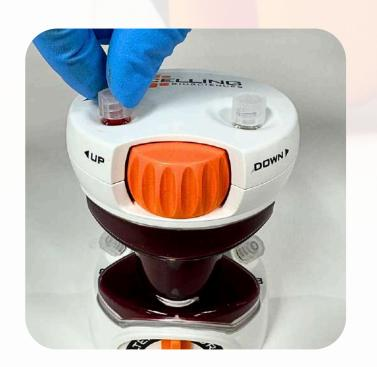
Remove the syringe and replace the cap on Port A. Ensure the collection window all the way up.
