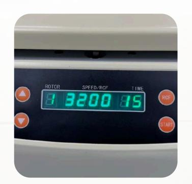
Centrifuge for 15 minutes at 3200 rpm. When spin cycle is complete, transfer the ART PRP+ to a flat working surface.
