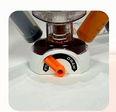
Adjust the flow valve to FILTER. A portion of the plasma will immediately be pushed through the filter when the lever is set into place.
