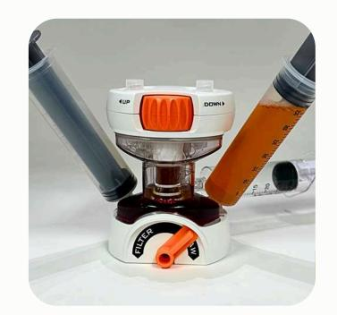
Slowly extract the aqueous plasma portion of the blood until air bubbles are observed in the syringe.
