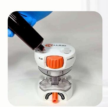
Connect the syringe containing blood to Port A by screwing it to the device.
