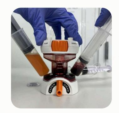
Quickly extract the buffy coat until air bubbles are observed.
