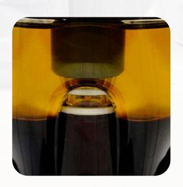
Lower the collection window until the bottom line of the lower ring is just above the buffy coat.
