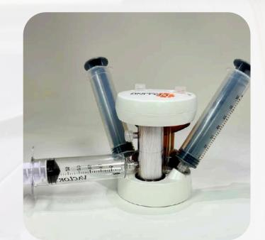
Unlock your syringes by pulling back on the plunger and pushing it back into place. Attach a 35cc syringe to Port B and Port C. Attach the VacLock syringe to the lower port of the back chamber. Pull the plunger all the way back and lock it into place.
