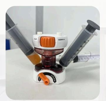
Attach a fresh 35cc syringe to Port B. Remember to unlock the syringe by pulling on the plunger and returning it back to its original place.
