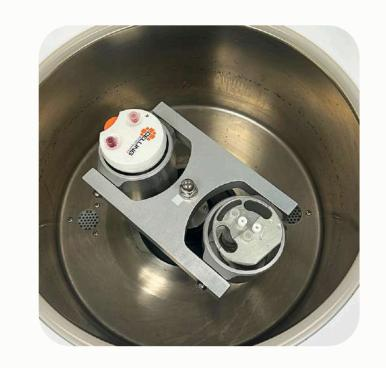
Load ART PRP+ into the centrifuge with the orange thumbwheel facing out. Ensure centrifuge buckets are fully seated. Use counterbalances as needed.
