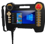
Uses touch GUI to train welders
