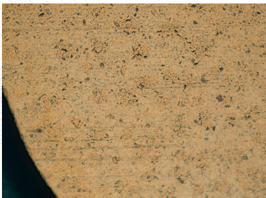
Figure 04: Stains after inadequate cleaning on PCB pad
