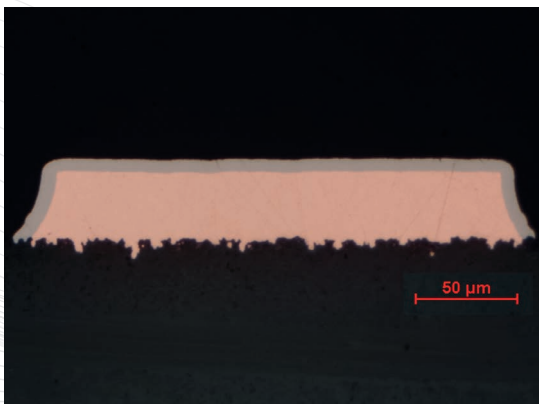
Figure 1: Cross-section of an ENIG coating system on a printed circuit board (Cu and Ni layers visible)
