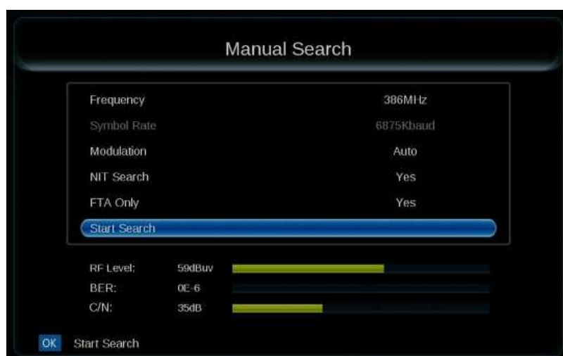
Fig. 21 — Installation menu > Manual Search
