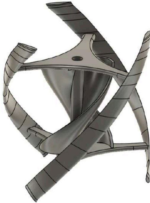
Fig. R2. CAD of 3D printed blades and 3D printed attachment to center.
