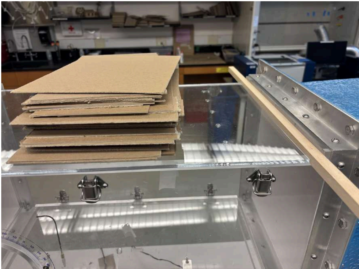
Fig. N1. Wind tunnel test section with lid and pitot tube access holes.
