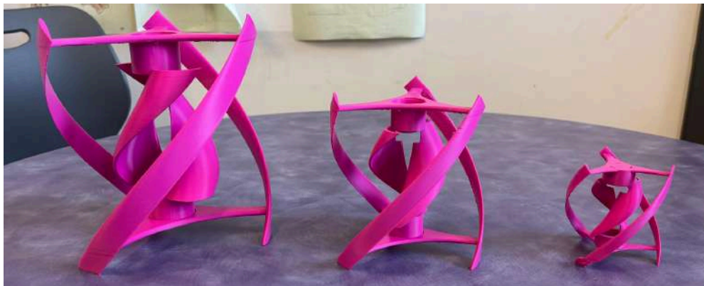
Fig. O1. The three prototypes used in scaling testing. From left to right the dimensions of the models are 7 x 6.3 in 2 , 5 x 4.5 in 2 , and 3x6.7 in 2 .
