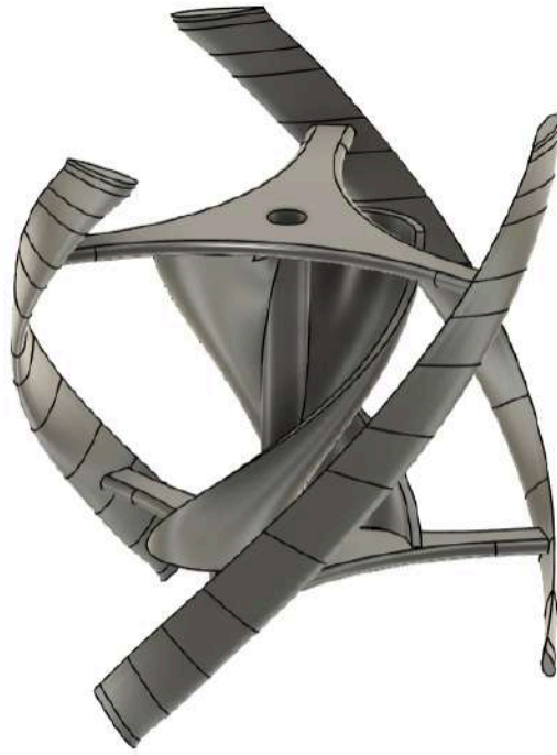
Fig. 23. CAD for 3D printed segment of full-scale VAWT.
