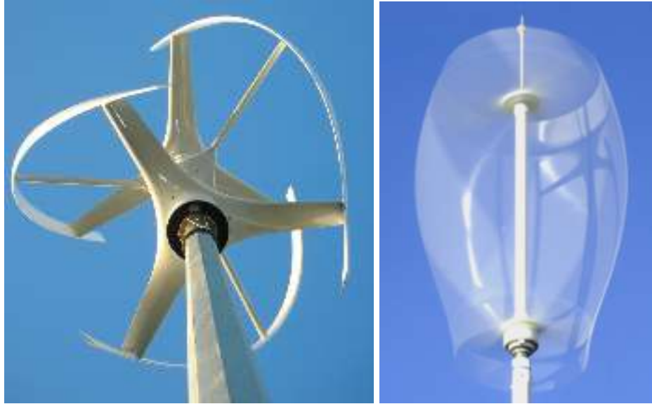
Fig. D1. Quiet Revolution Qr6 Vertical Axis Wind Turbine static (left) and in motion (right). adapted from [D2].
