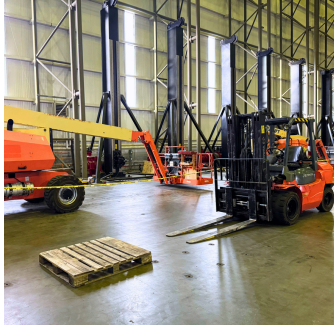
Forklift and Boom-lifts
