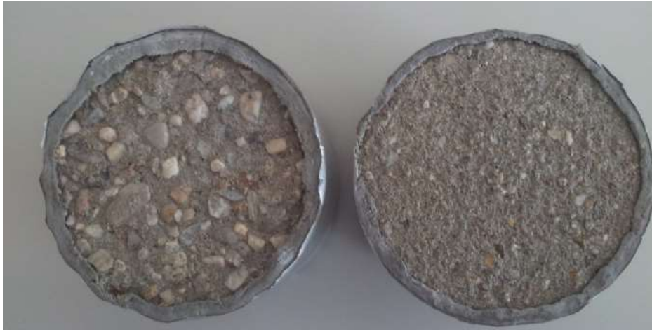
Image 2 : Right the concrete surface treated with RC M040, left the untreated concrete surface.
