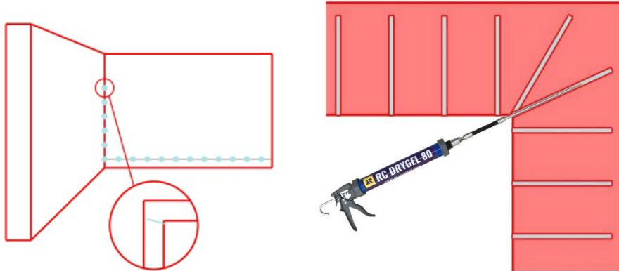
Between injected walls and adjacent interior walls that do not require treatment, a vertical layer of RC DRYGEL 80 must be applied. Respect a minimum height of 120 cm and a minimum of 50 cm above the highest rising level of the wall moisture and the salts. Inside corners must be drilled diagonally, distance between the holes: 10 to 12 cm.
