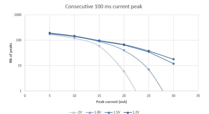
The graphs above illustrate that the battery can sustain multiple successive current peaks, confirming its ability to deliver high power consistently. Even under repeated stress, the battery's performance remains stable, and its power capabilities can be leveraged multiple times consecutively without the necessity for immediate recharge. This behavior is particularly advantageous for applications requiring frequent, short bursts of high current while maintaining operational continuity
