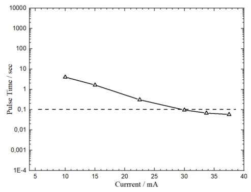
The battery can deliver currents far exceeding 200C (e.g. > 30 mA) for sub-100 ms pulses without triggering voltage collapse or thermal limits.
