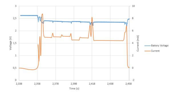
Despite the current peaks associated with radio transmission, the battery exhibits only minimal instantaneous voltage drop and maintains stable output. This ensures the system can support hundreds of transmission events before requiring a recharge.
