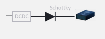
Figure 20: Reverse current protection with Schottky diode
