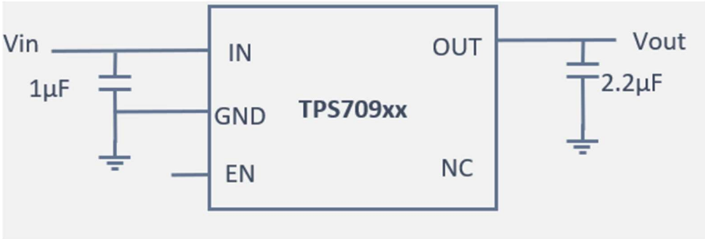
Figure 4: Schematic of TPS70927 (TI) Fixed 2.7V output voltage, LDO voltage regulator
