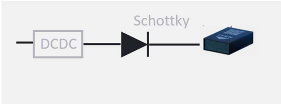
Figure 20: Reverse current protection with Schottky diode
