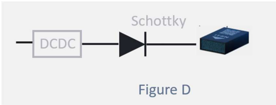
Figure 24: Reverse current protection with Schottky diode
