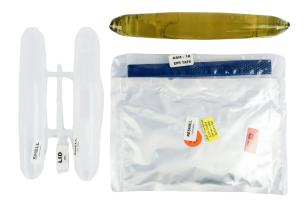
ARJP...CL / CRJ...ES low-voltage resin straight-through joint and splicing kits are designed for connecting PVC and XLPE cables. The two-component, flame-retardant clear epoxy resin remains flexible, offering superior insulation and water-blocking properties.
