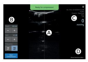
The screen shows: a) the ultrasound signal with a vertical line, b) the buttons for manual adjustment of the ultrasound image depth,
