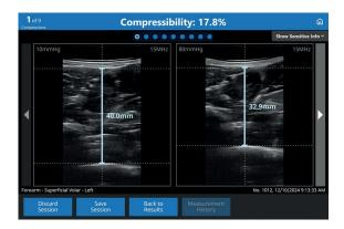
The compressibility percentage ("CP Value") indicates in % by how much the compartment had been compressed at 80 mmHg relative to 10 mmHg and is thus a measure of the relative compressibility.
