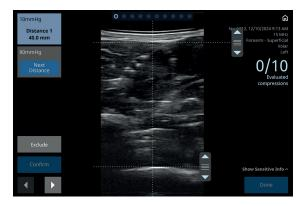
Once the landmarks are placed for 10 mmHg, the user can proceed to the 80-mmHg compression by tapping the grey 80 mmHg selection button. On the 80 mmHg picture, the measurement is performed in the same way as at 10 mmHg.
