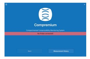
The CPMX1 System will become operational by pushing the power button on the Tablet. After the CP Software has been fully loaded, the start screen will show two buttons: "Start" and "Measurement History". The current software version is shown on the bottom-right corner of the screen.
