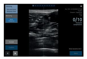
For the measurements of interest, the user locates an outer landmark, e.g. external fascia, and marks it with his finger by tapping on the screen. A transverse line is placed automatically for its identification on the screen.
