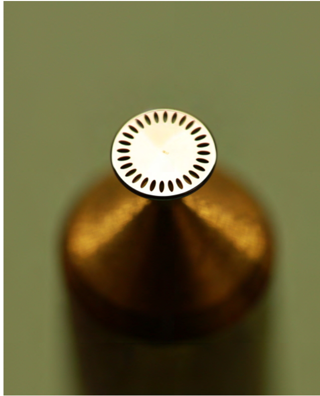
Figure 4: Combined optical-THz resonator made of silicon. THz frequency modes are guided by the petal structure of air holes; these holes were cut by femtosecond laser machining.
