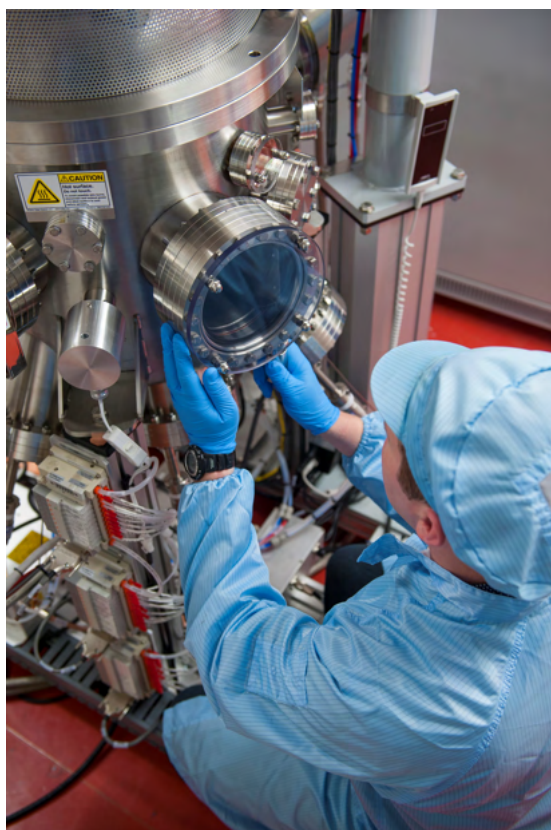
Figure 3: Checking the operation of an ultra-high vacuum chamber for magnetic thin film growth at VUW.
