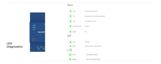
The IoT LED must remain constantly on. When it is transmitting, it flashes at a 10Hz rhythm. If the LED is not constantly on, no additional participants are found in the network. The Run LED indicates whether connected sensors are detected, which could be a SMARTenergy sensor or MBus/Modbus participants. The LTE LED blinks to indicate the availability of an LTE network. If it remains ON continuously (for at least 30 minutes), an external antenna must be used.
