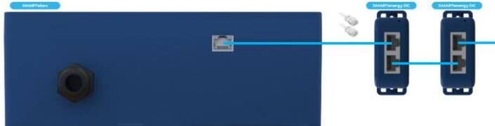
The SMARTenergy sensors DC are connected to the SMARTebox via standard RJ45 network cable AWG27. For looping through the signal, 2 RJ45 sockets are provided on each SMARTenergy sensor.
