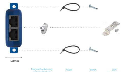
The following options are available on the SMARTenergy for mechanical installation:
