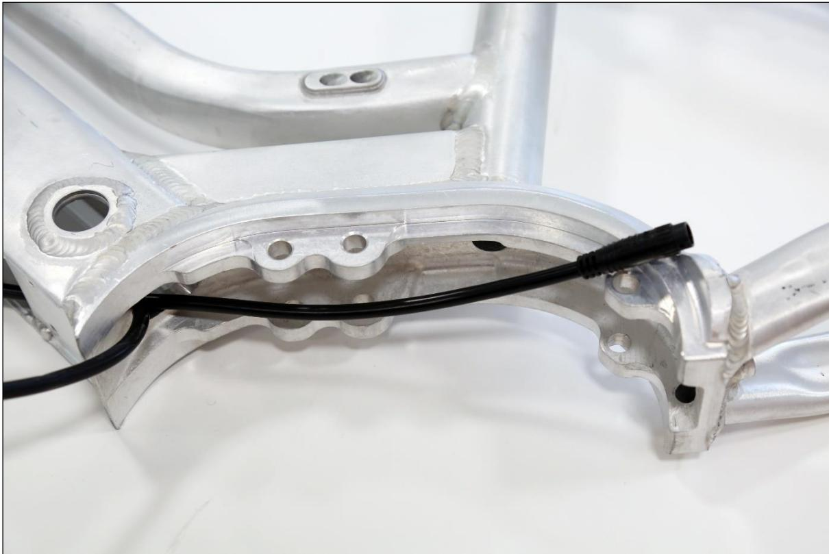
Connect the wire to the center motor.
