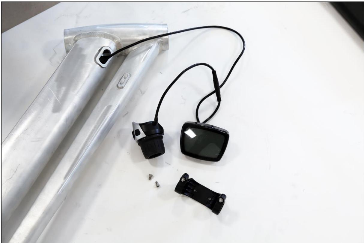
Mount the bracket onto the display.
