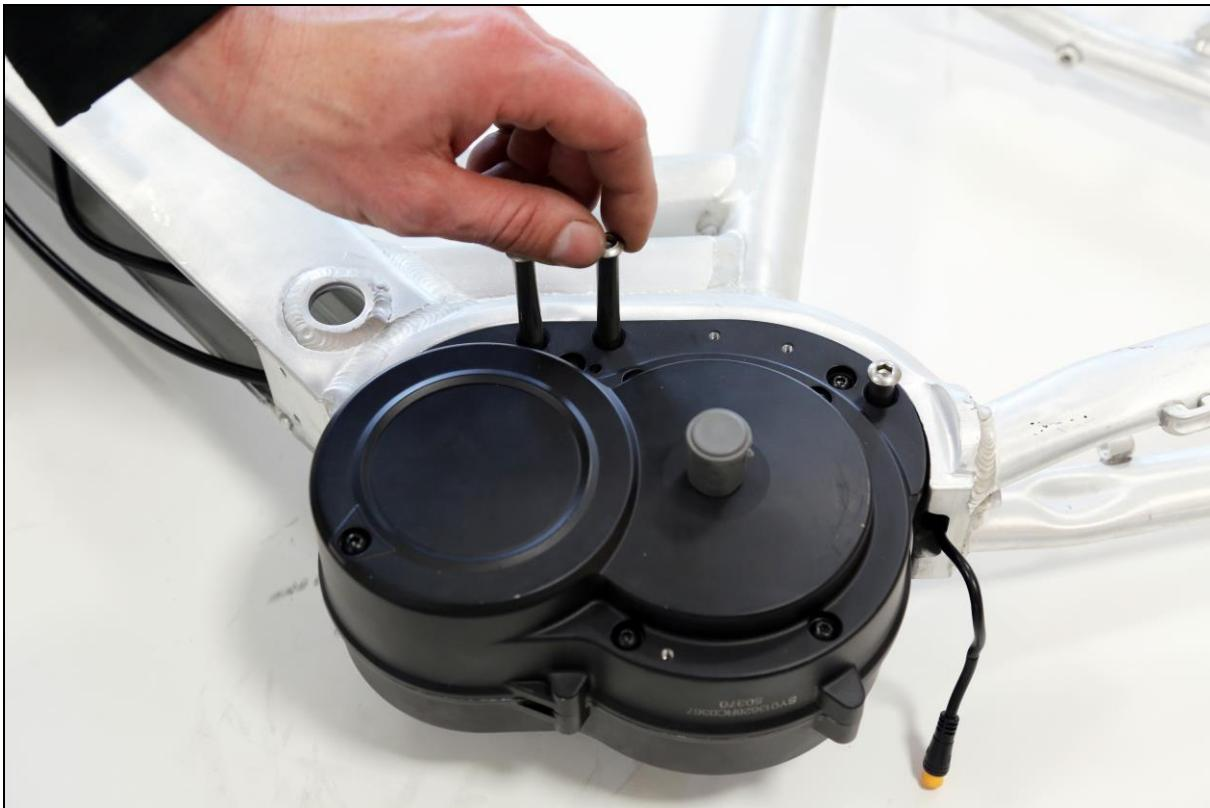
Tighten the three M6x18 screws (6Nm) for the center motor.
