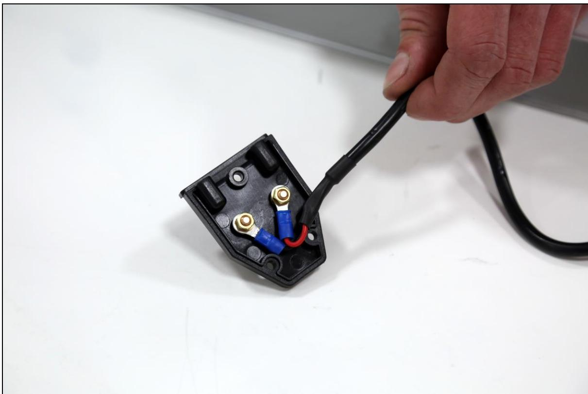
Tighten the front to the backplate using the three M3x10 screws (1.2 Nm).
