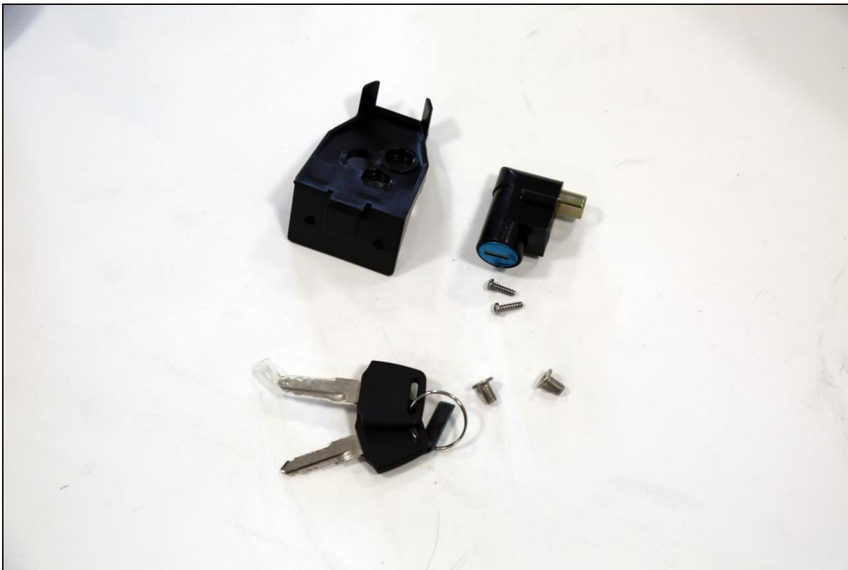
Mount the two screws loosely and make sure the key part can move around.
