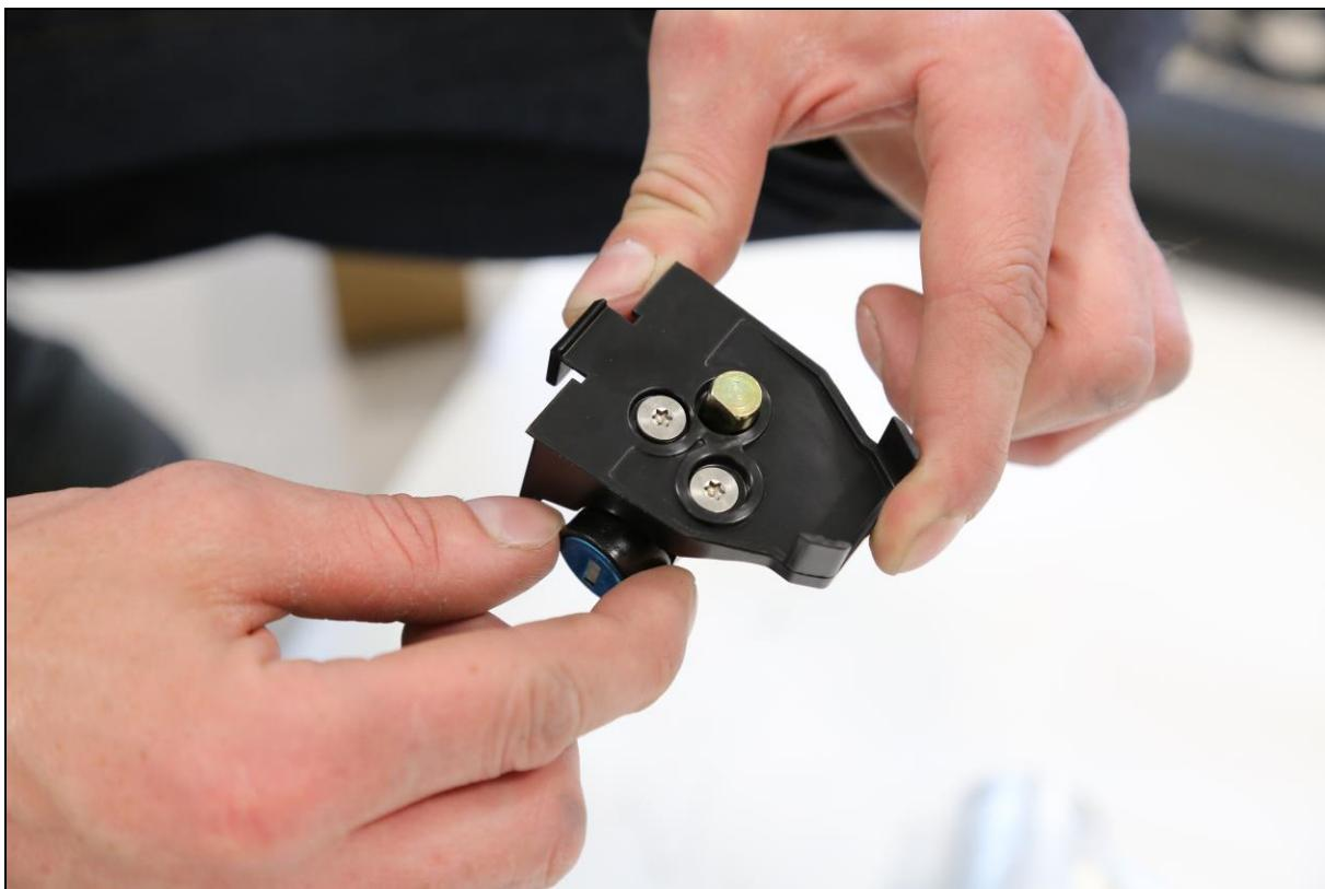
Push the locking mechanism in place. Make sure the wires are positioned correct.
