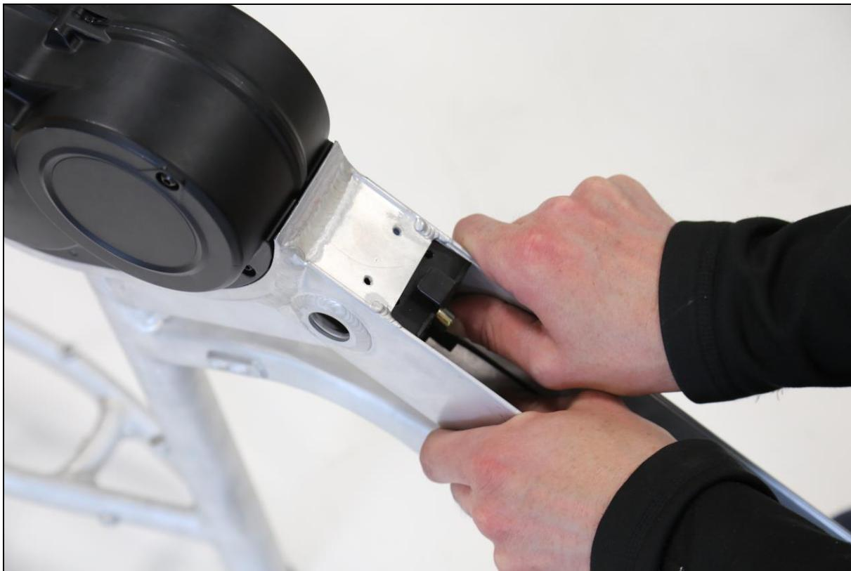
Fit the key into the lock to use it as a guide while fitting.
