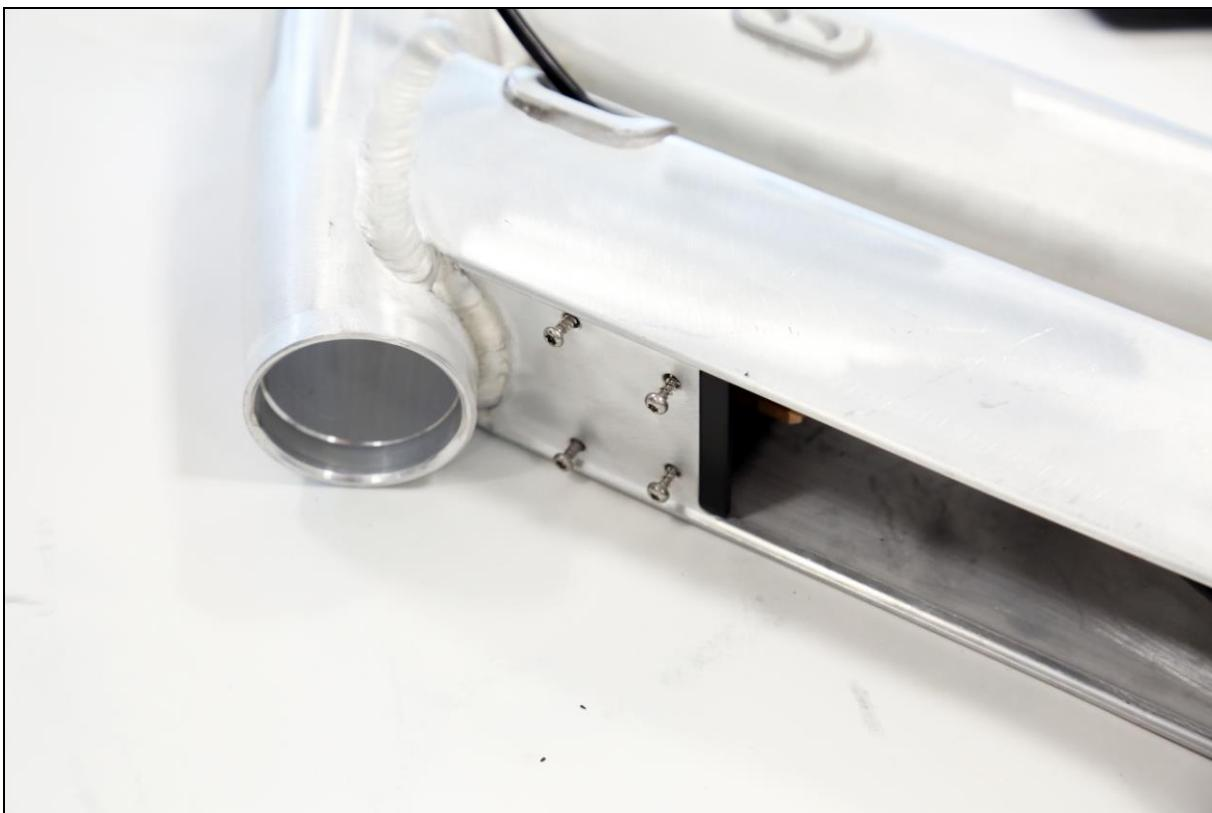
Put the wire from the socket box hub into the lower hole of the downtube.
