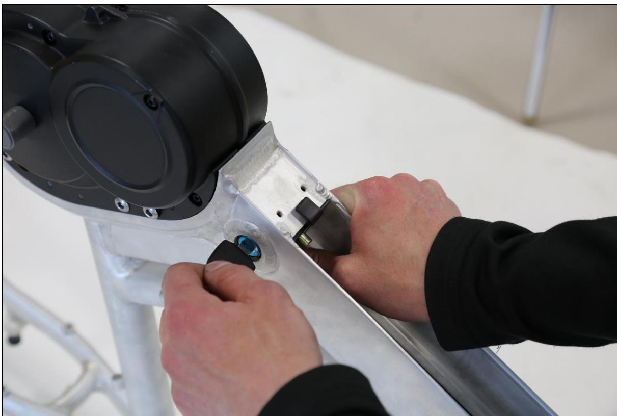
When in place tighten the two M3x10 screws (1.2Nm).
