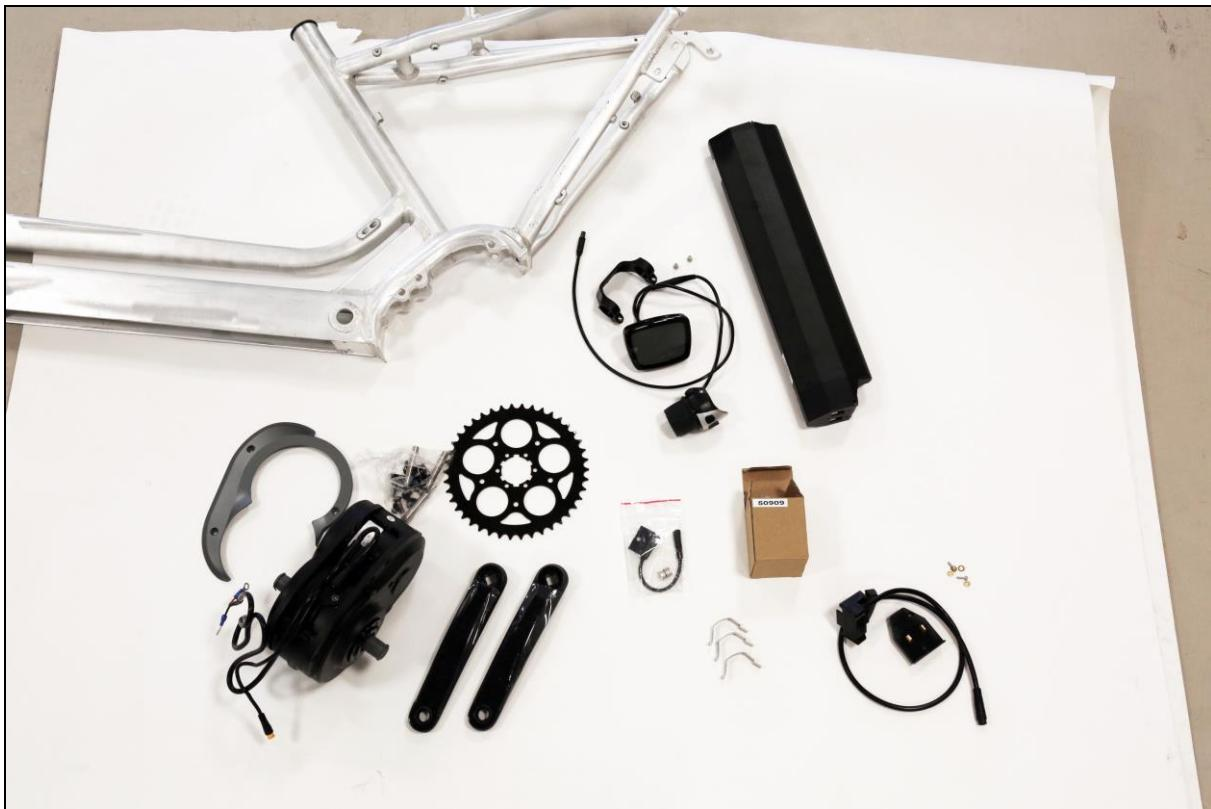
Start by taking the frame and center motor. Run the power wire from the motor thorough the hole into the downtube.
