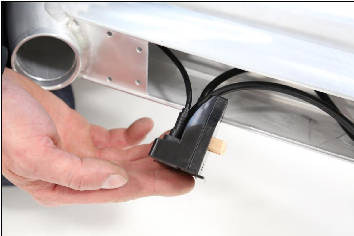
Fit the socket box hub into place. **IMPORTANT:** make sure the wires are guided on each side of the socket box hub.
