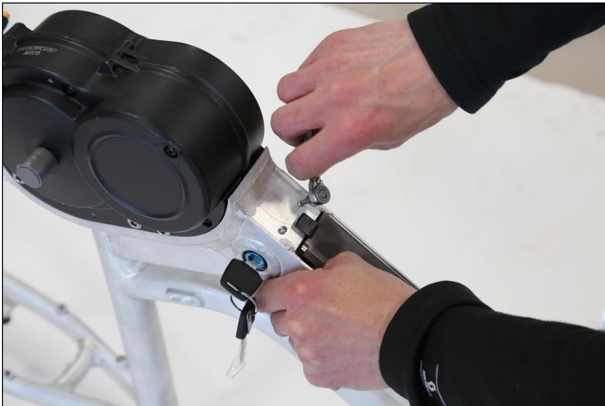
You may now tighten the two screws for the lock (1.2Nm)
