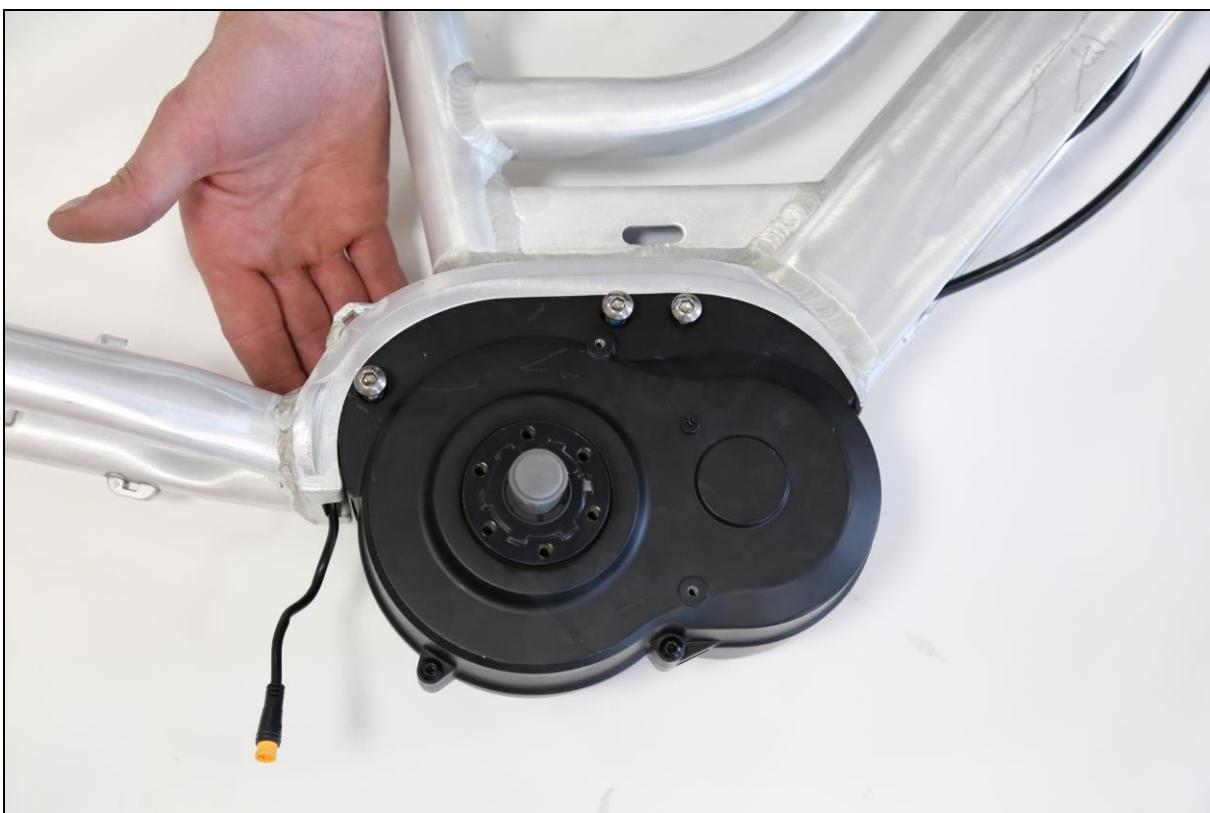
Turn the frame and run the wires in each side. Fit two of the three clamps – one close to the socket box hub and one in the middle.
