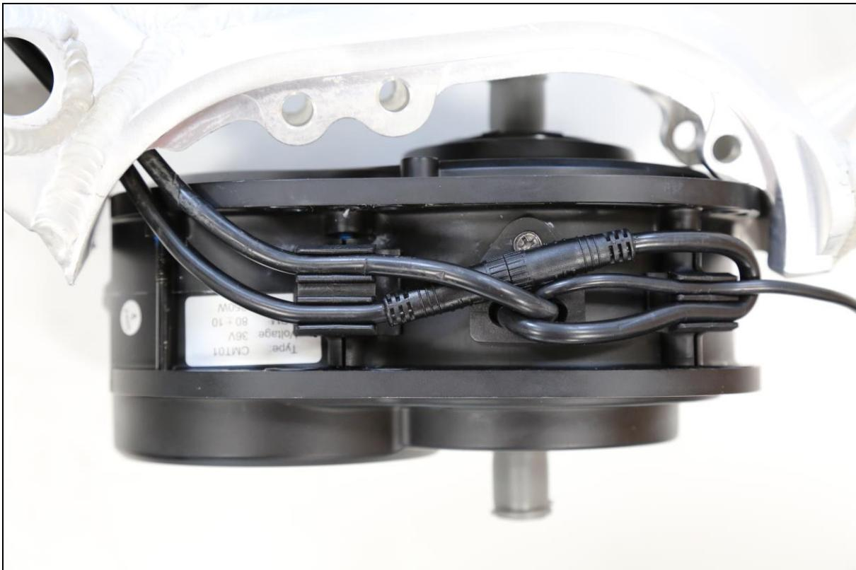
Fit the screws for the center motor.
