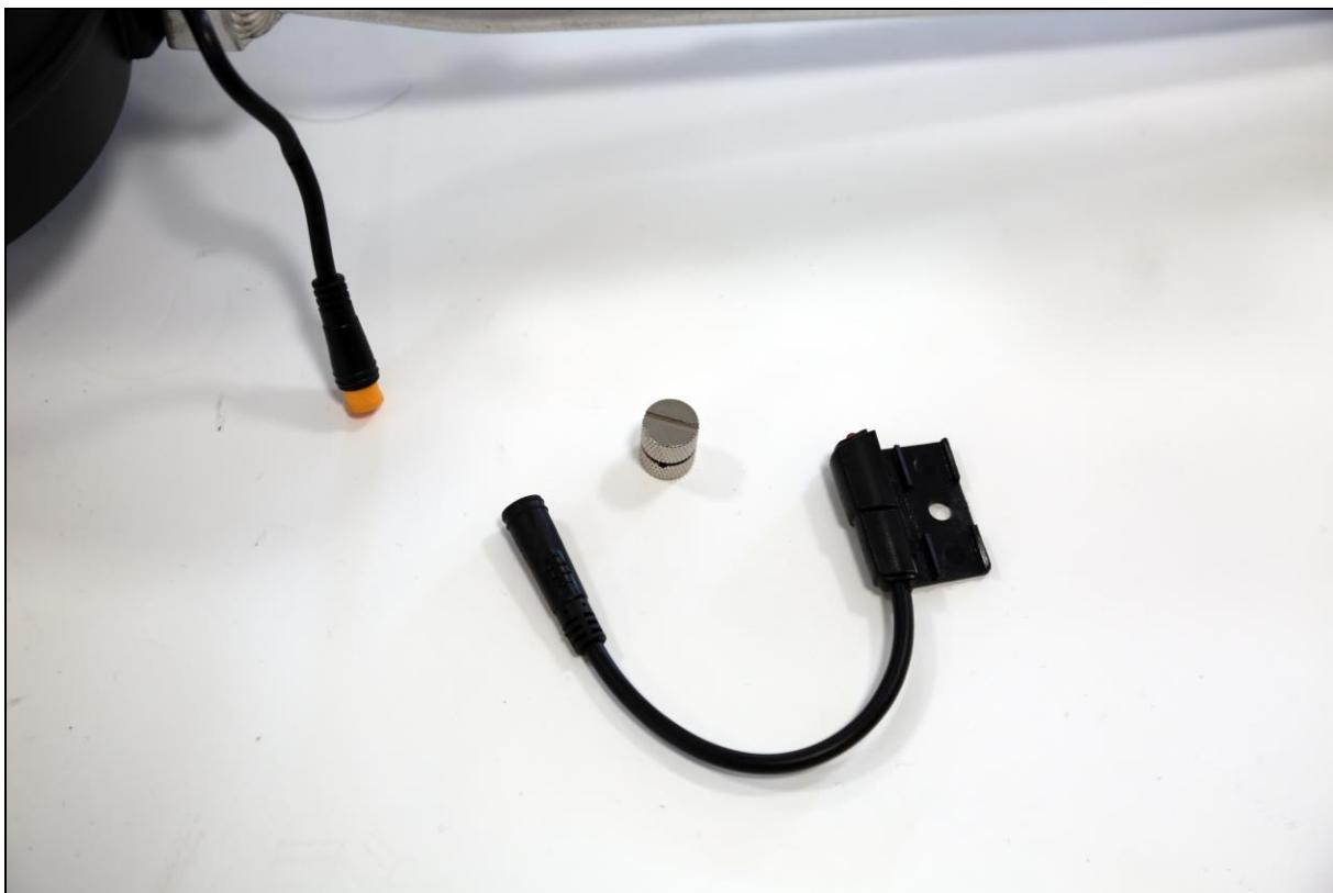
Connect the wire from the sensor to the motor and mount the speed sensor onto the frame.
