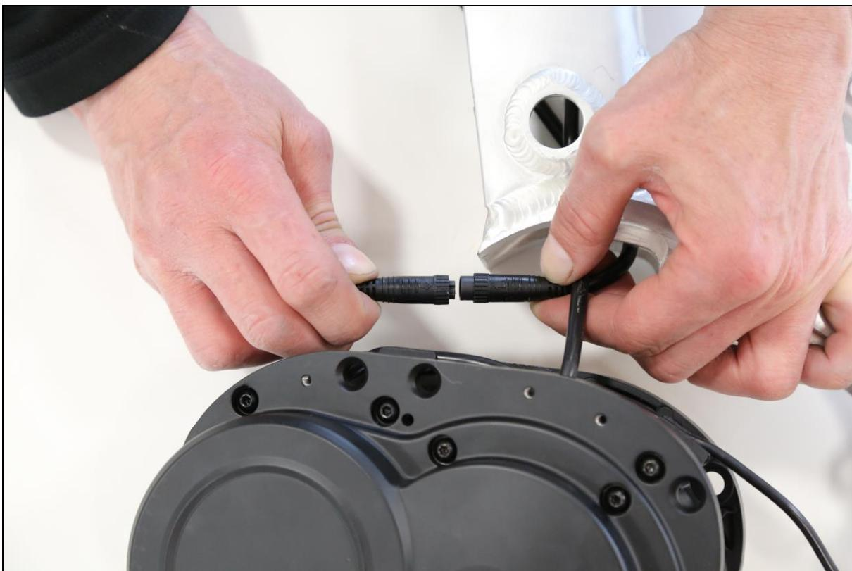
Make sure the wires are positioned like this and fit the center motor to the frame. Make sure the speed sensor wire doesn't get stuck.
