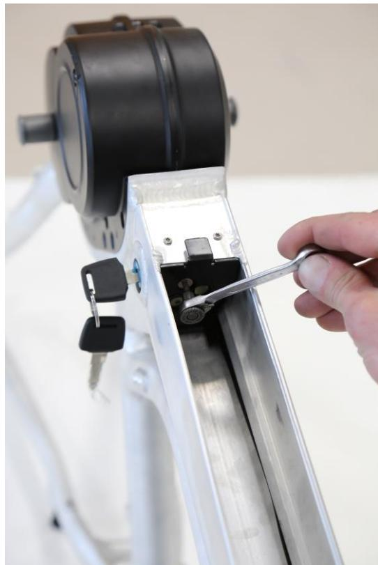
Fit the last clamp closest to the locking mechanism.
