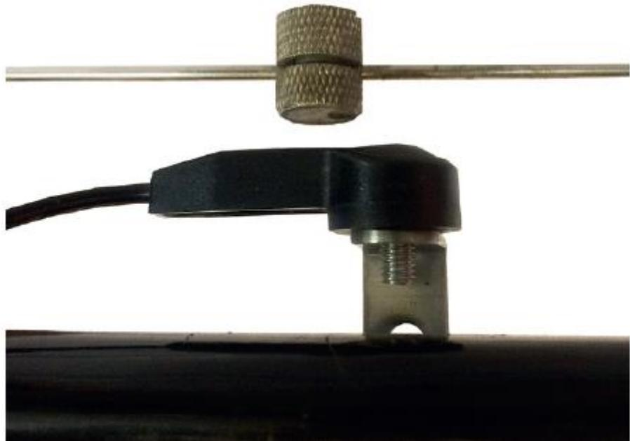
Test the bike, if the error code number 7 is shown adjust the speed sensor
