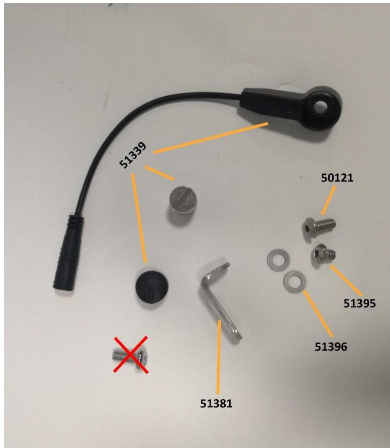
Assemble the speed sensor in the order as the picture (bracket, speed sensor, washer and screw)
