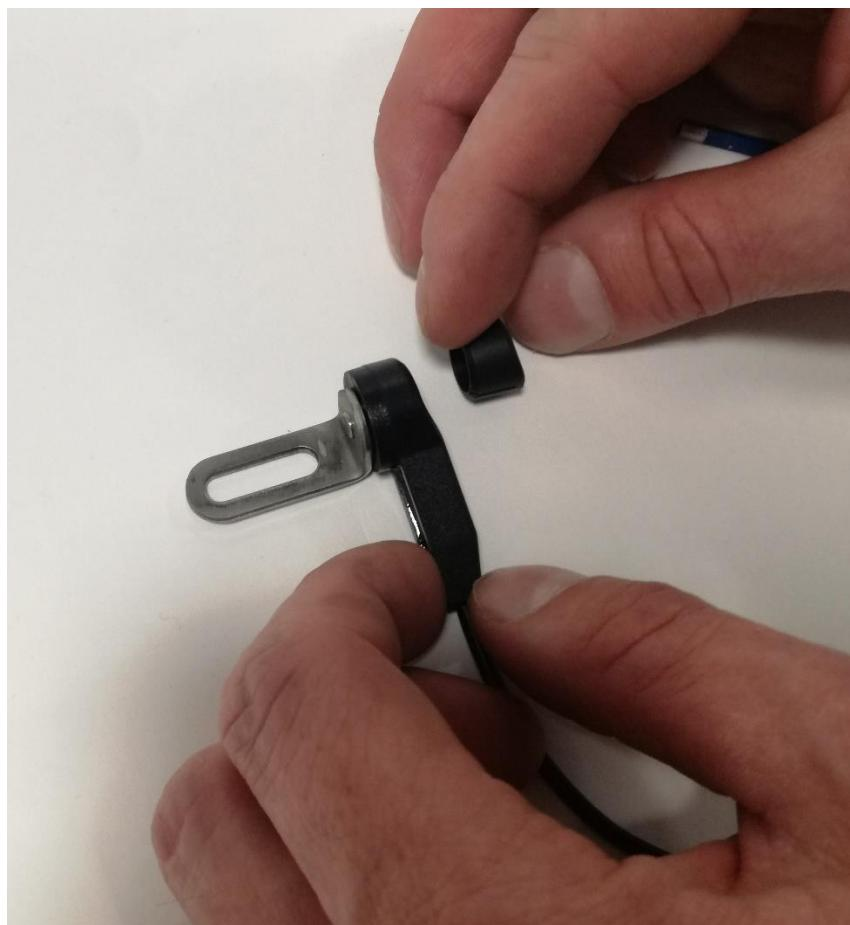
Mount the speed sensor to the frame.
