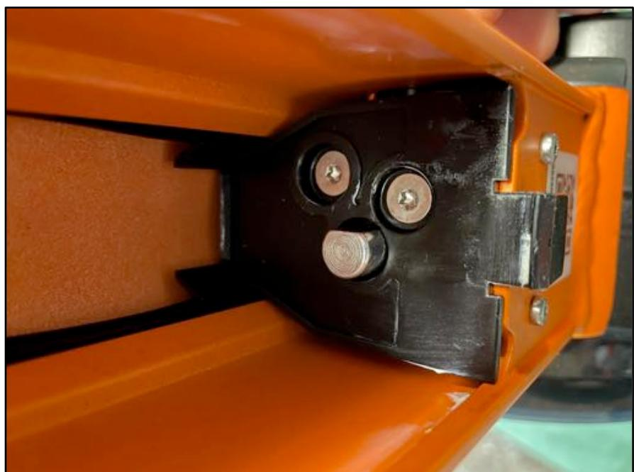
3. When fitting the battery ensure that it has been pressed into the frame completely.
