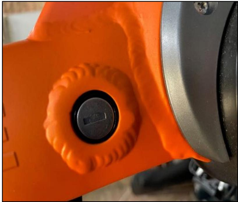
5. If the key does not turn freely when locking the battery into the bike you will need to loosen the 2 x T15 torque head screws and change the position of the lock.
