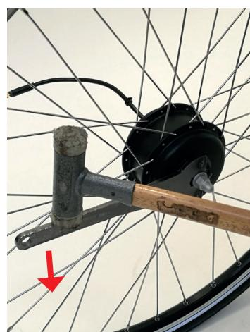
Mount the special tool on the lid with disc and nut.
