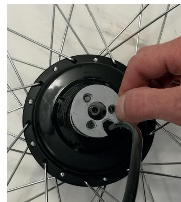
Hold on to the shaft with 10 mm wrench and loosen
