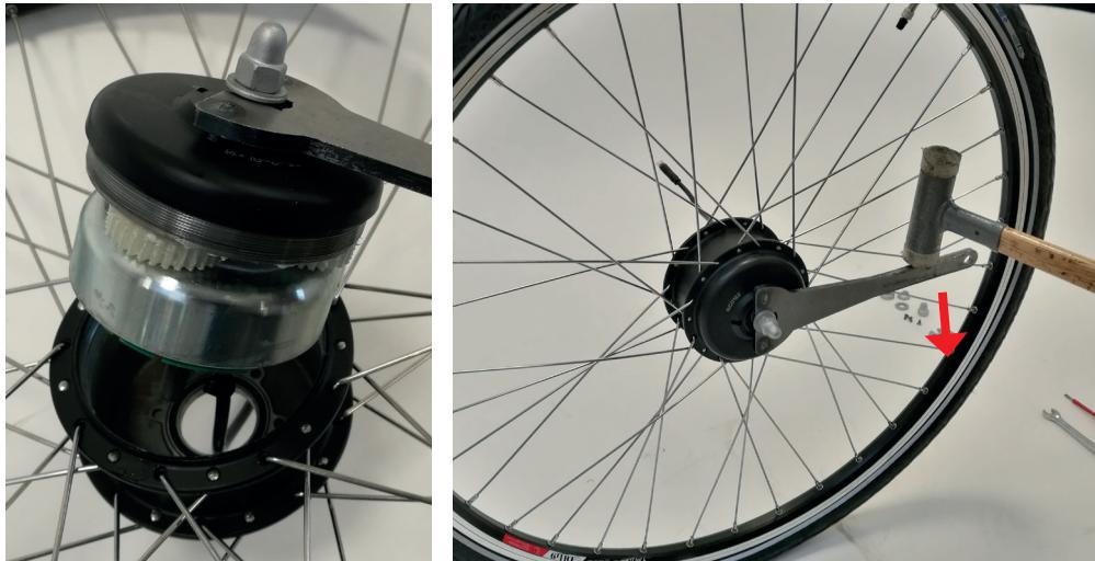
Fit the innerpart of the motor housing.
