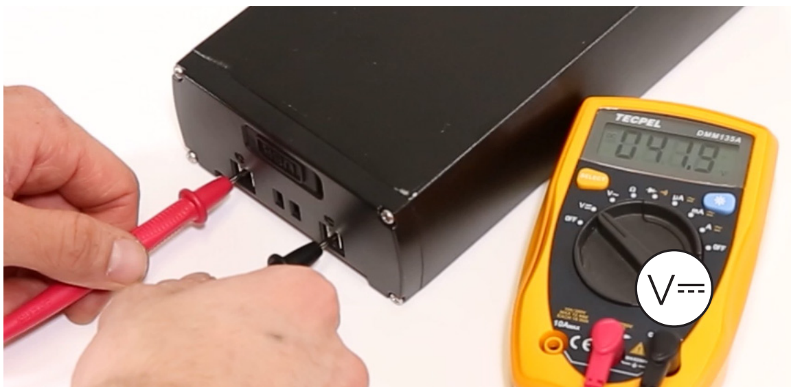
Picture 1: Set the voltage meter to DC-Voltage and measure the battery. When a battery has been fully charged the battery must measure at least 41.3 V.
