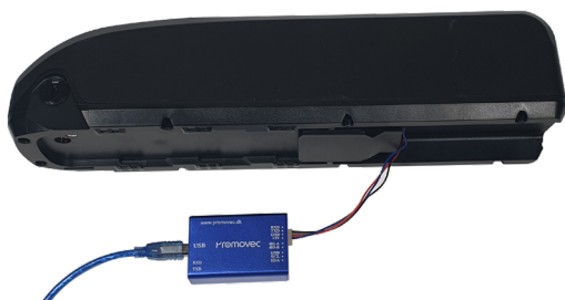
Read out adaptor for Downtube 2 XL connected to the USB outlet on the blue read out tool
