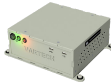
PowerCube: Powerful small form factor PC with shock mounting options.
