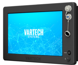
All-Weather: IP67/IP68 weatherproof computers and monitors for outdoor use.
