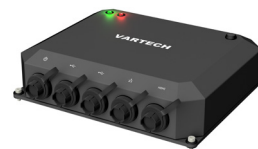
ToughCube: Fully sealed small form factor computer for 24/7 operation.
