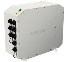
Bolt (Ai): Fully sealed, weatherproof edge AI computer designed for outdoor operations.
