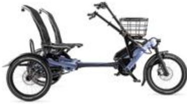
Figure 4: Fully suspended parallel tandem for two: The Kettwiesel TWO by Hase Bikes
