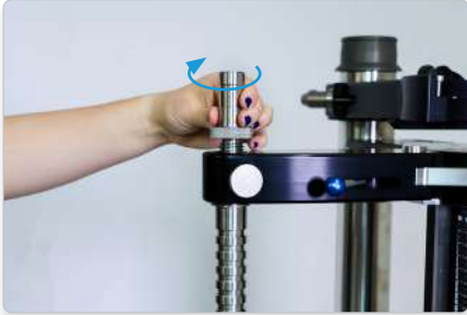
Screw on 25mm pin adapter (314453).
