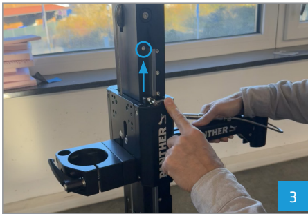
Flip Quick Lock and push the sledge upwards until it locks in.
