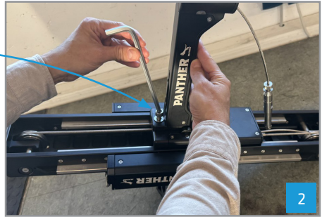
Unfold the arm and tighten the marked screw.
