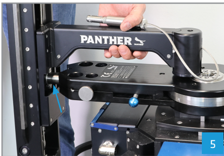
Insert the marked bolt into the hole, but not completely. IMPORTANT: The column must be fully retracted.
