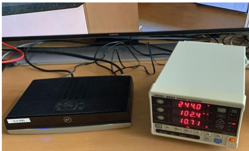
Current Approach to Power Consumption Measurement: Lab Sample Testing
