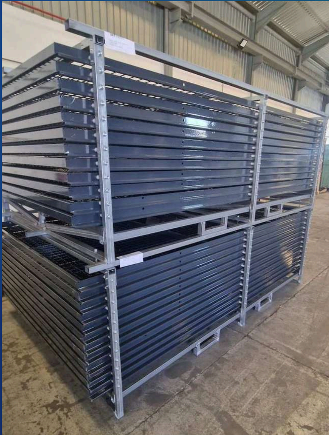
MESH are separated & 100% protected during transportation Avoid scratch, repair & future rust
