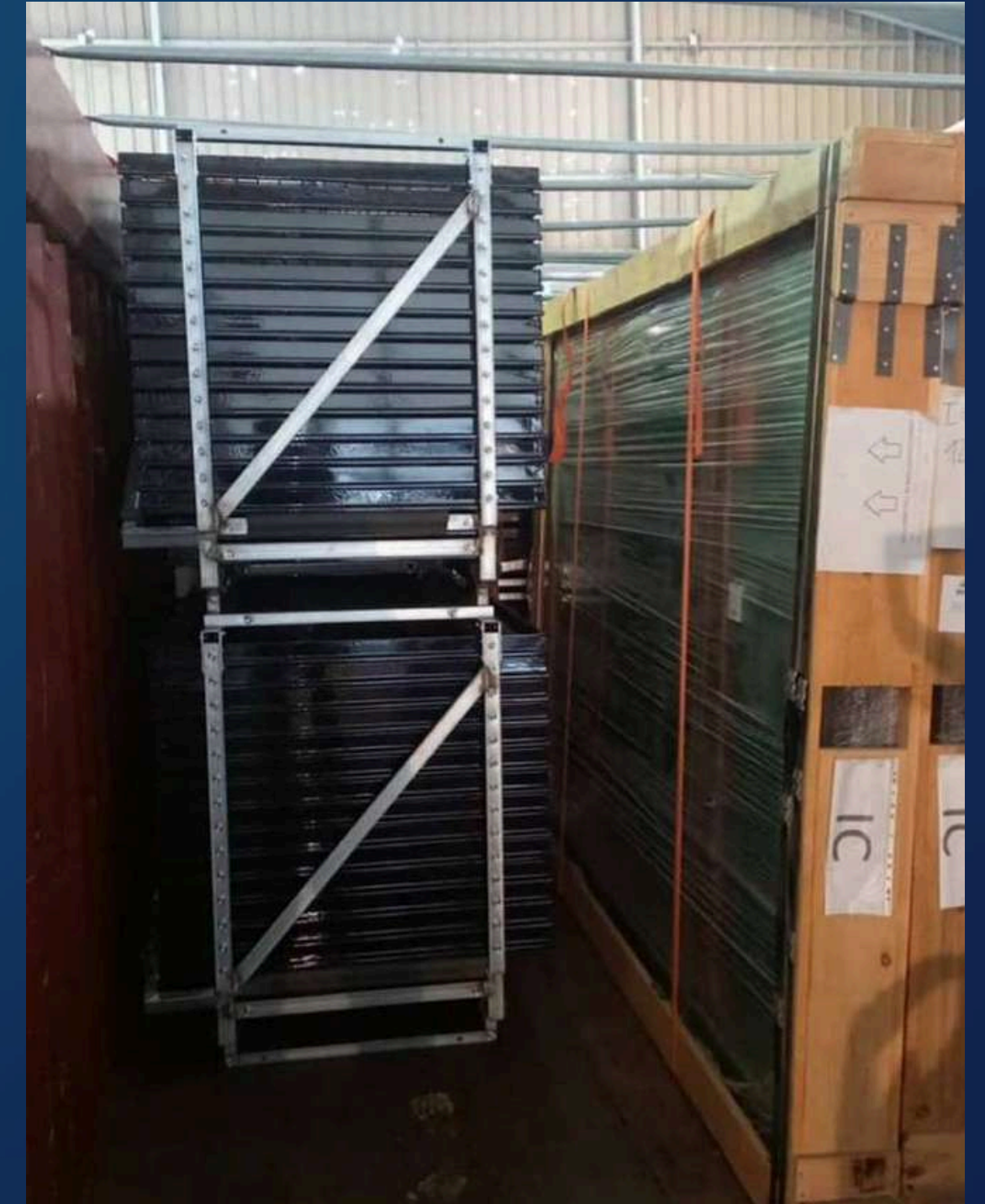
Into the truck/container, material are separated, protected and tied. Avoid damage during transport
