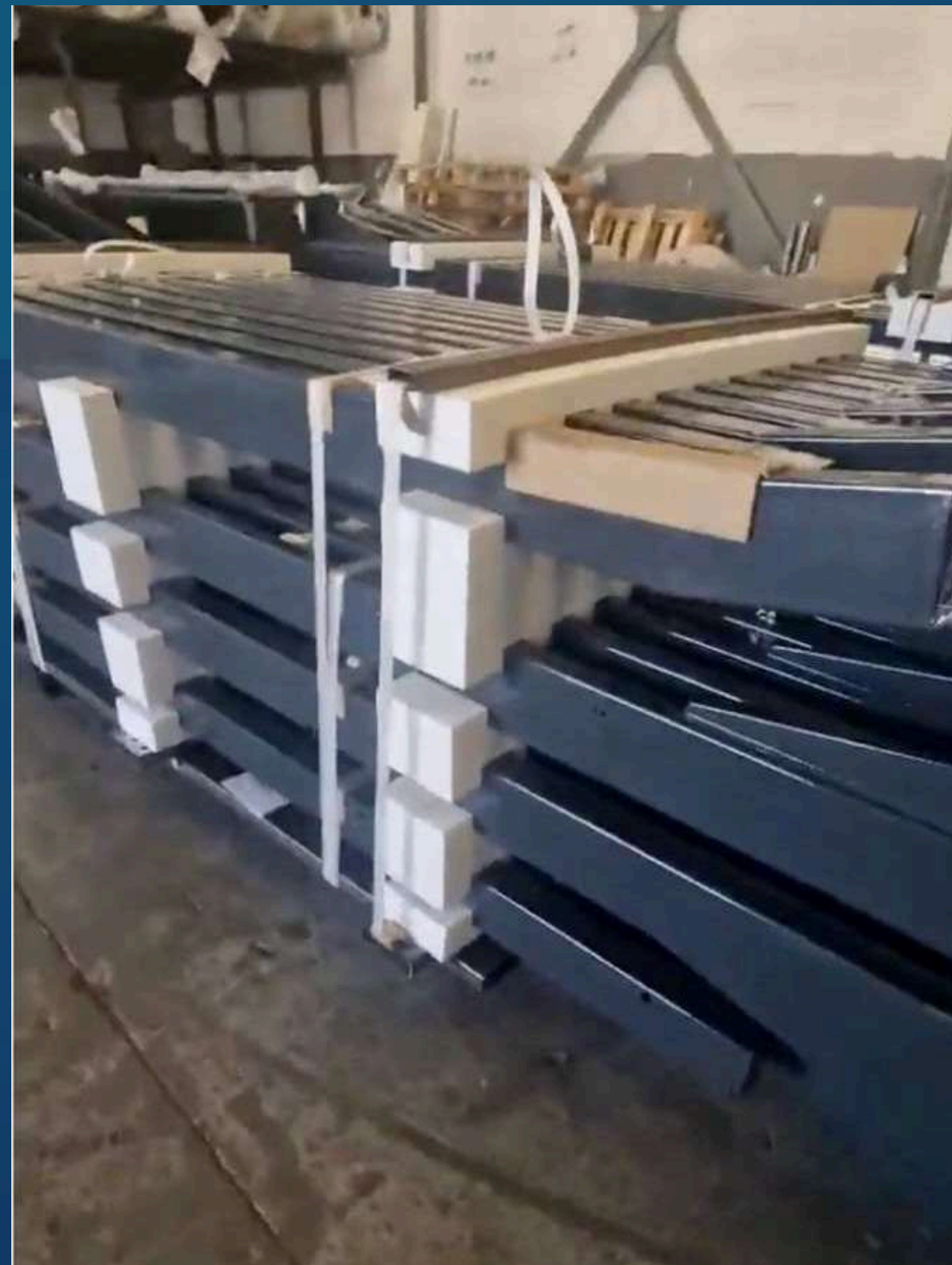
POST are separated and 100% protected during transportation Avoid scratch, repair & future rust
