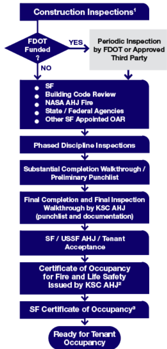
Figure 4: CCSFS Construction Inspection Process
