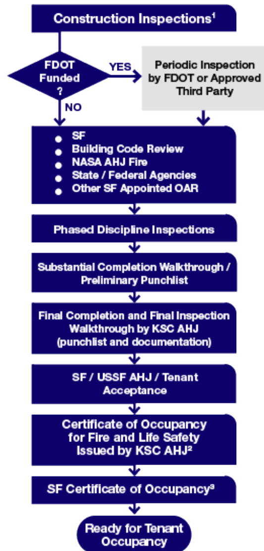
Figure 5: KSC Inspection Process
