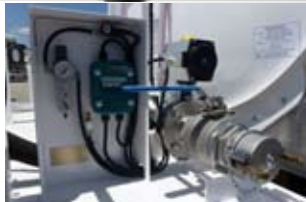
Liquip MPP102 tank monitor system for overfill protection
