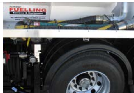
Fitted with vapour recovery system
