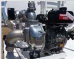
Yanmar L70 with electric start and centrifugal pump.
