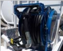
Spring rewind hose reel with 20m x 25mm hose & nozzle
