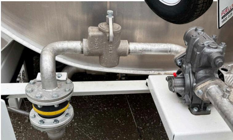
Haar 38mm vane pump with bypass valve, Epex basket type suction strainer. All 316 Stainless pipe & fittings
