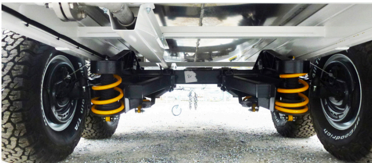
Heavy duty Simplicity suspension.
