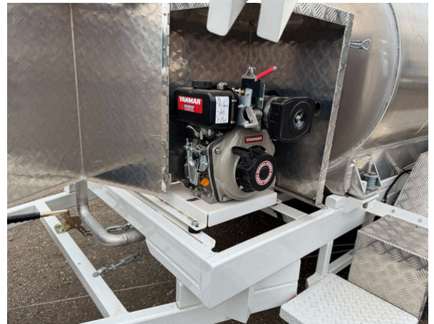
Yanmar L48 diesel engine powered pump. Engine fitted with flame arrestor exhaust and mechanical engine strangler for emergency shut down.
