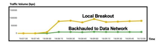
The figure shows the traffic behavior over time, comparing Local Breakout versus Backhauled to Data Network. The graph highlights that local breakout traffic (yellow) significantly outpaces backhauled traffic (green), showing the efficiency gained through traffic offloading.
