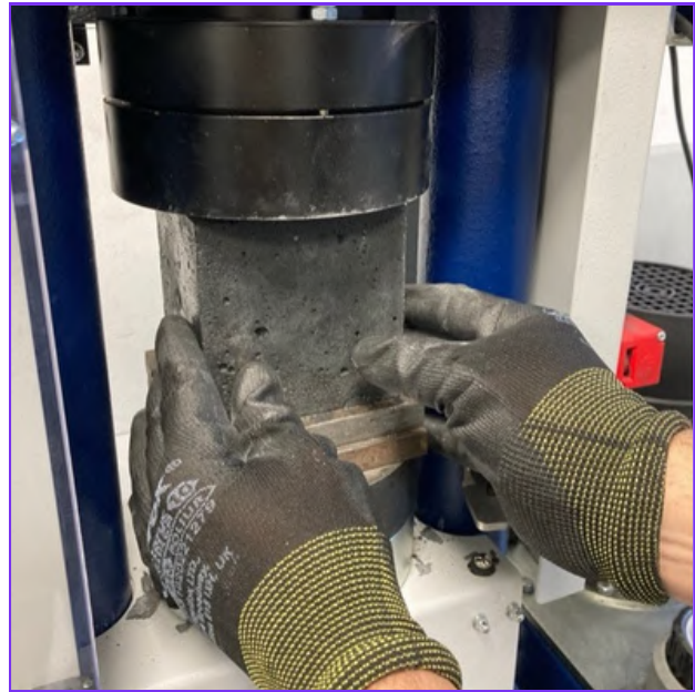
Caption: A biochar-concrete block is being tested for compressive strength. Image used with permission of ecoLocked GmbH.
