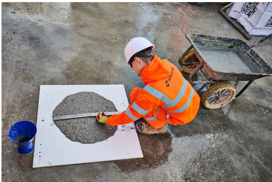
Caption: An engineer is conducting a slump flow test on a biochar concrete mix. Image used with permission of Holcim.
