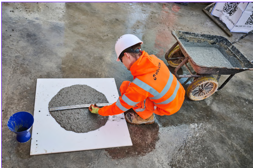
An engineer is conducting a slump flow test on a biochar concrete mix. Image used with permission of Holcim.
