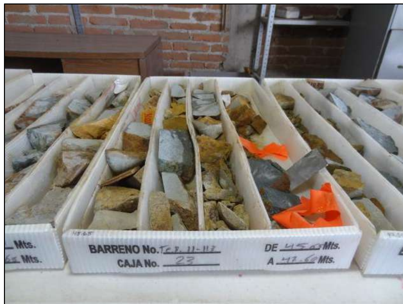
Figure 12.6 A View of Some Core Boxes for Drill Hole TEP-11-113
